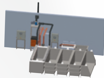
▲ Electropolishing plant with a container size for part lengths up to max. 3,000 mm
