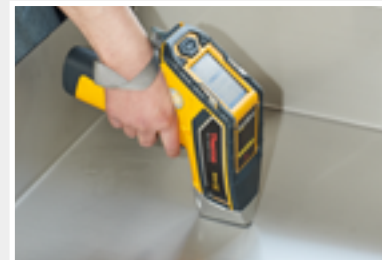
▲ X-ray fluorescence measuring device for material identification
