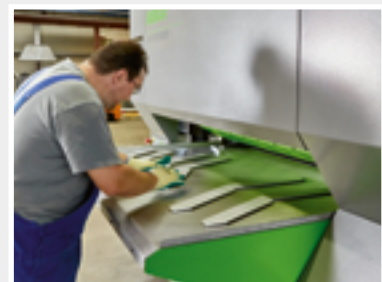
▲ Straightening machine for the straightening of sheet metal
