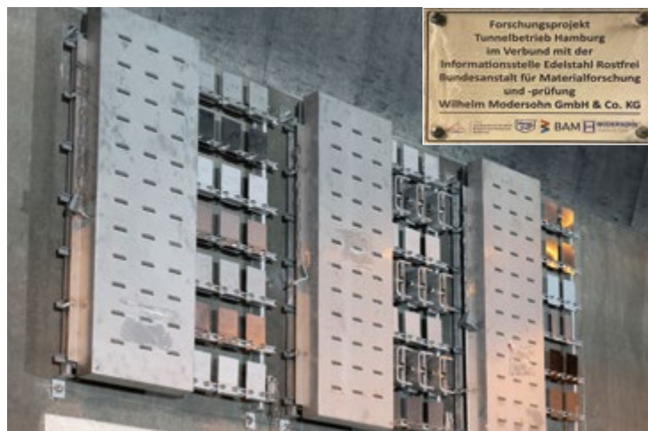
▲ Installation of the material samples in the Elbe Tunnel Hamburg, as part of a research project to expand the application range of the material 1.4462.
