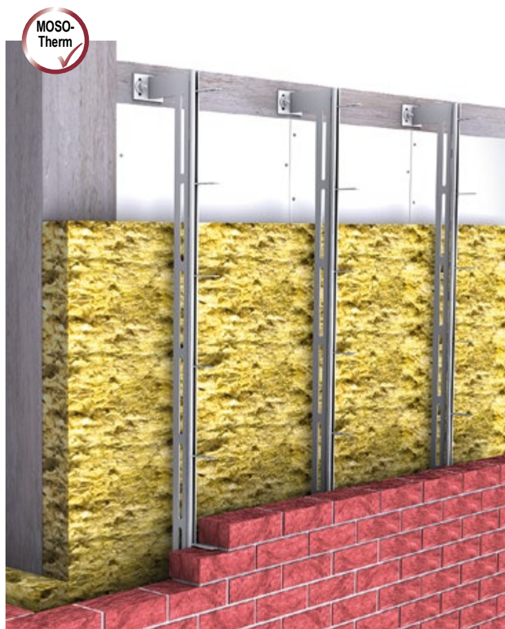
▲ Anchoring with MOSO® wind post anchor HV-WP
