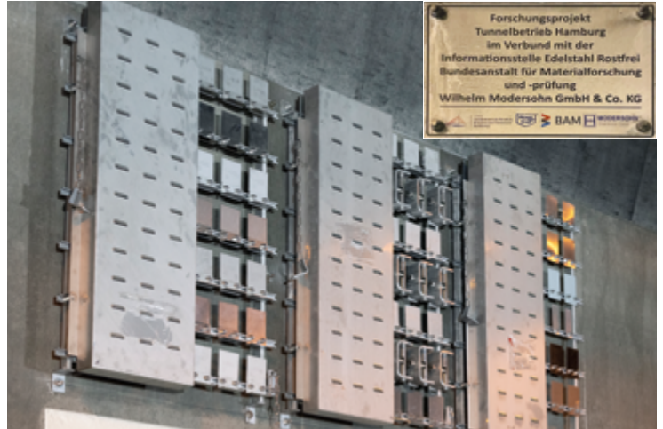
▲ Installation of the material samples in the Elbe Tunnel Hamburg, as part of a research project to expand the application range of the material 1.4462.
