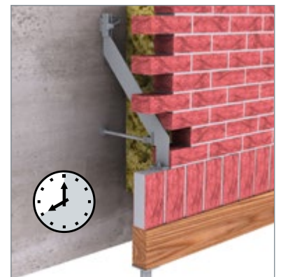
▲ Only remove local supports once the masonry mortar has completely hardened!
