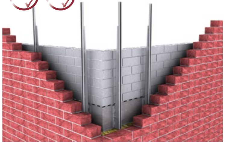
▲ Fascia anchoring with MOSO® horizontal connection HV-A
